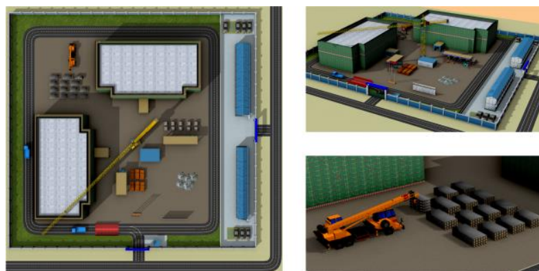
Figure 18. The layout of prefabricated components on the construction site.
